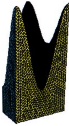
Fig. 11 Typical tetrahedral mesh for a unit corrugation three-dimensional wavy surface ( \tau=0.8 , Re=125 )
