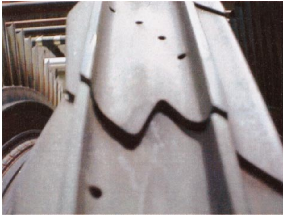
Fig. 7 Shroud mismatch after 48,000 hours
